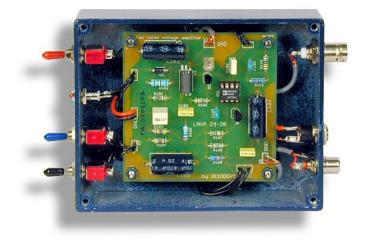
On the receiver are placed the Gain Control: 0, 12 and 24 dB, for best matching aerial antenna or short wip with the audio card sensitivity. A low pass filter with frequency cut over 100 Hz has been added, to give better conditions when you use this device for very low frequency signals reception, like Schumann resonances.
