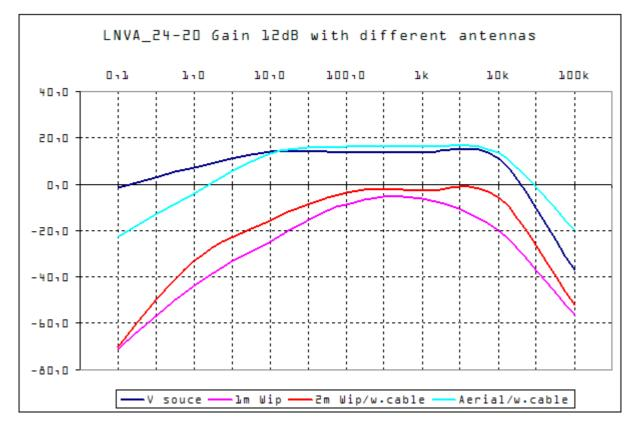
Here there are the characterization curves of the LNVA\_24-20 set with gain of 12 dB with different antennas.
