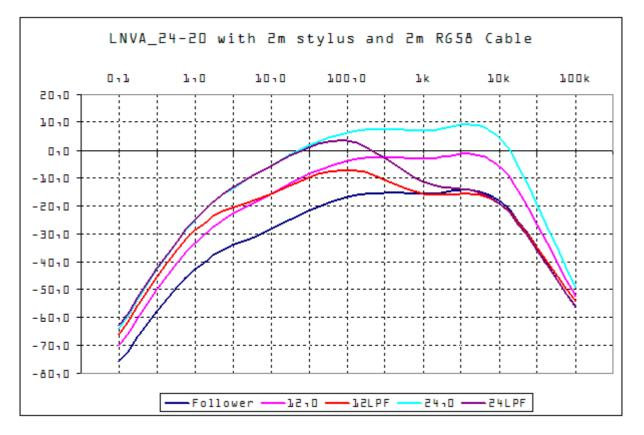
Here there are the characterization curves of the LNVA\_24-20 using a 2m stylus connected with 2m of RG58 cable to the receiver. Measures have been done in a reason of a 30 pF equivalent stylus capacity and 195 pF from cable.
