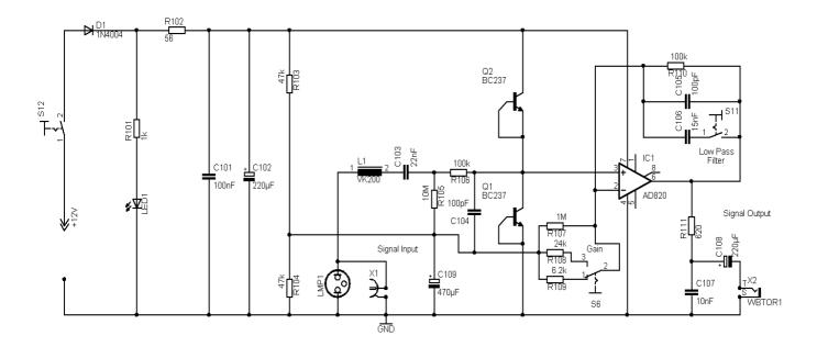
This is the simply electric schematic: the core of the circuit is the AD820, the operational amplifier of Analog Device with a very low noise current of 0,8 pA. This circuit performs, coupled with the 10 MOhm input resistance, a really very low noise amplifier device, with a noise figure better than 0,1 dB.
