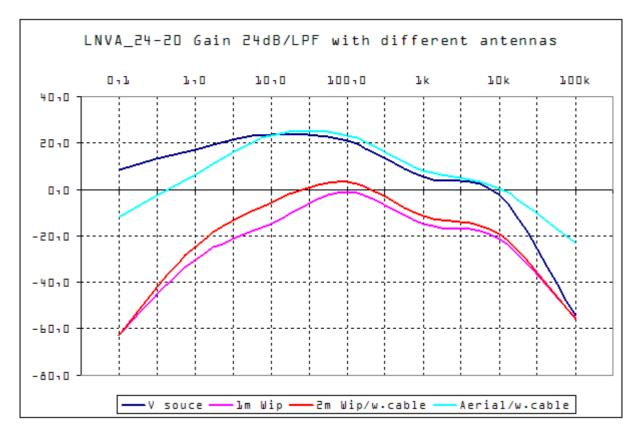
Here there are the characterization curves of the LNVA\_24-20 set with gain of 24 dB and 100 Hz low pass filter with different antennas.
