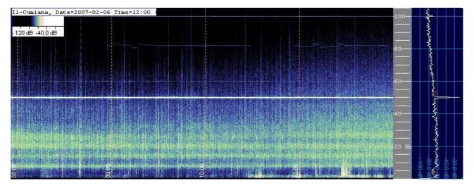
This spectrogram reports a reception with a 45m long wire, connected to the LNVA\_24-20 with 50m of RG58 coaxial cable. Schumann resonances are clear and strong, as for the two pattern of 82 Hz submarine signals.
