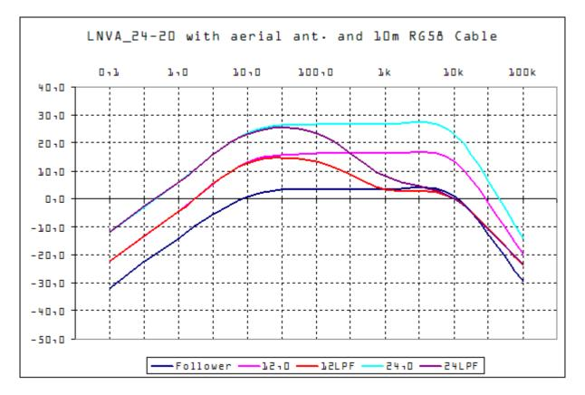
Here there are the characterization curves of the LNVA\_24-20 using an aerial wire antenna connected with 10m of RG58 cable to the receiver. Measures have been done in a reason of a 195 pF equivalent antenna capacity and 1000 pF from cable.
