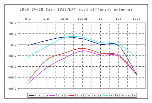
Here there are the characterization curves of the LNVA\_24-20 set with gain of 12 dB and 100 Hz low pass filter with different antennas.
