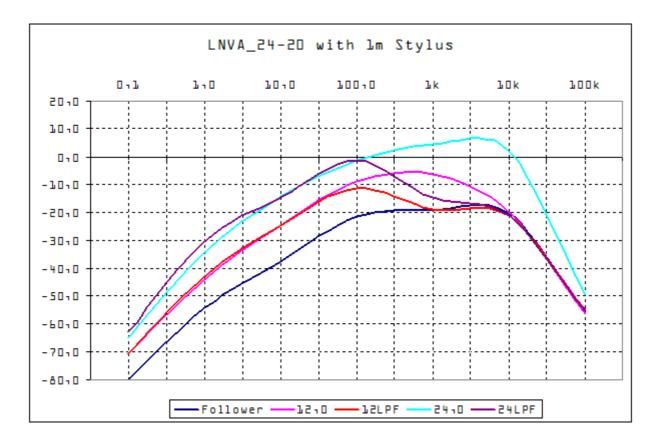
Here there are the characterization curves of the LNVA\_24-20 using a 1m stylus placed directly on the receiver. Measures have been done in a reason of a 18 pF equivalent capacity.
