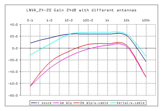
Here there are the characterization curves of the LNVA\_24-20 set with gain of 24 dB with different antennas.
